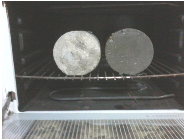
Figure 3: Drying specimens in oven for absorption test.
