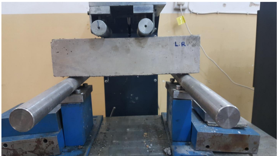
Figure 2: Concrete beam under testing for flexural strength.
