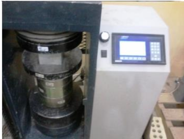
Figure 2: Beam and cube specimens under testing for flexural and compressive strength
